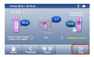
ATTENTION, when an incubation time is required, you must observe it and you cannot exceed it for more than 30 seconds in order to obtain a valid result. Always ensure you have performed this step properly before proceeding to the next step.
